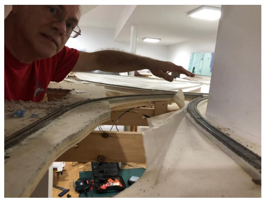
I added some supports underneath to hold the cut-out. Over the homasote, I'll use Gaterboard as the base for whatever structures and scenery I use there, making sure the Gatorboard is larger than the cutout it will sit upon. Needless to say, it would have been MUCH Better to do this before I laid track and did wiring.
